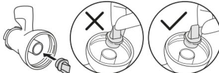
**4** Attach the pump body to the bottle.
